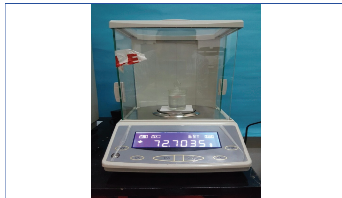
[Table/Fig-2]: An electronic balance device with four digit precision.
